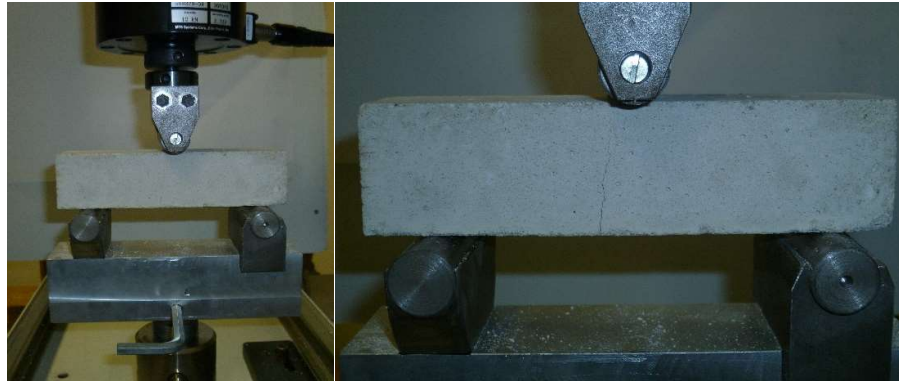
Figure 2:3: Test setup in the laboratory for determination of flexural strength of mortar.
