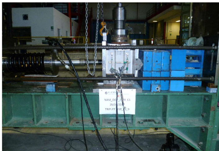
Figure 2:26: Test set-up in laboratory for evaluating the shear strength of masonry joints.
