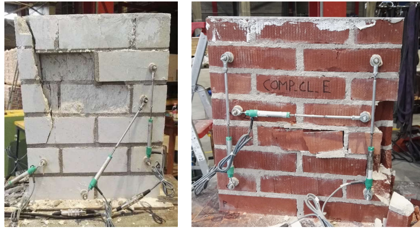
Figure 2:17: Failure of CS (left) and clay (right) wallette under compression perpendicular to bed joints..
