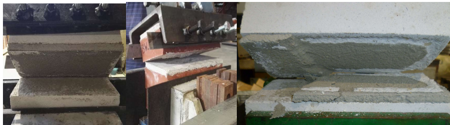
Figure 2:38: Example of failure modes from bond wrench tests in the laboratory.
